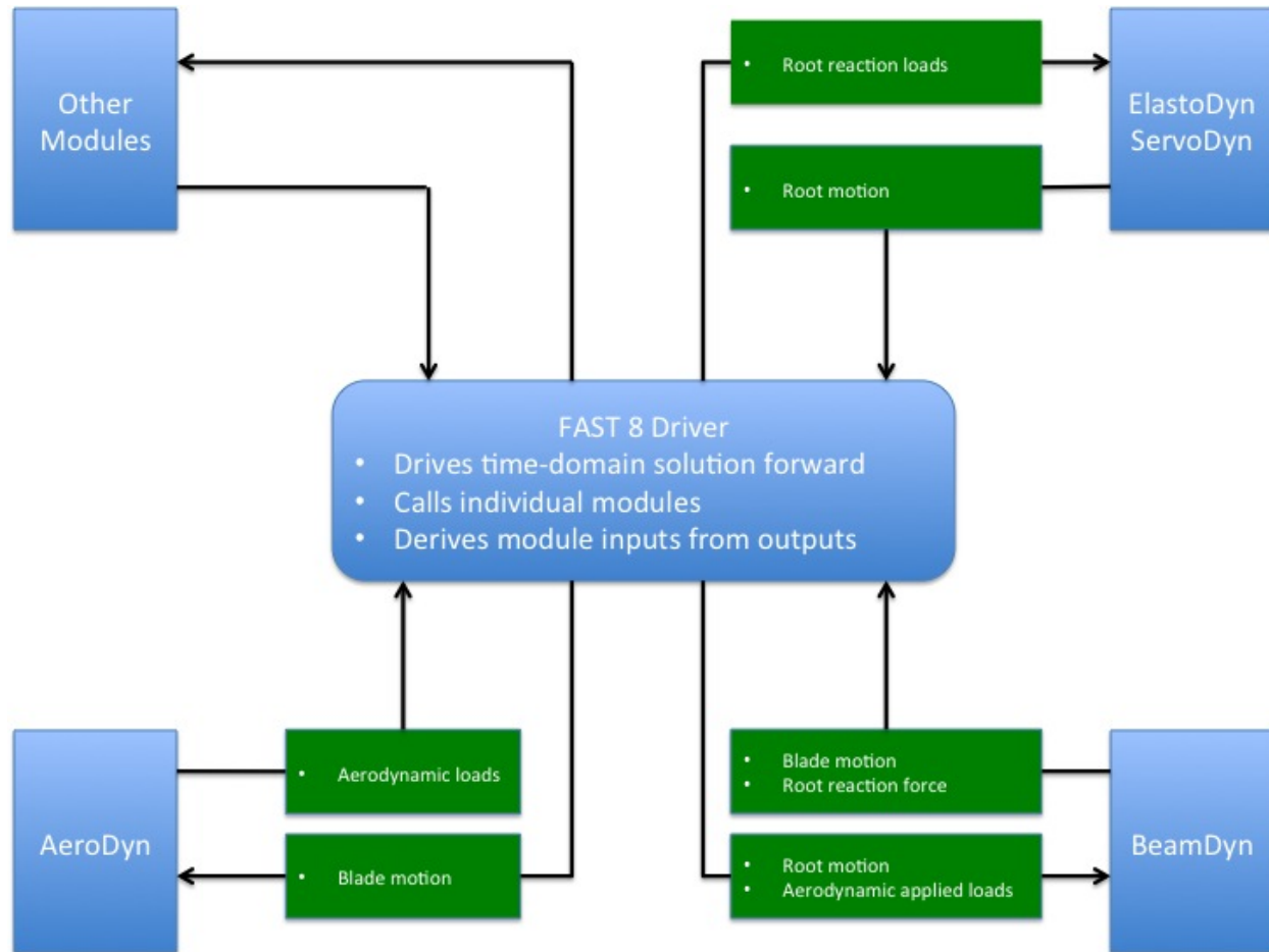
Fig. 4.24: Coupled interaction between BeamDyn and FAST
